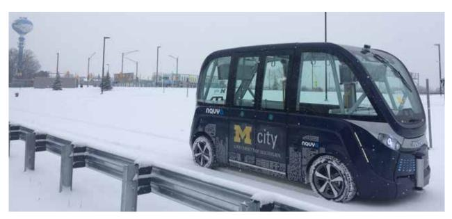
Mcity evaluated the performance of a NAVYA driverless shuttle for over a year in a variety of weather and lighting conditions inside the Mcity Test Facility.
