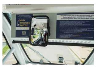
A mirror located inside each shuttle helps the on-board safety conductor see what's happening behind them.
