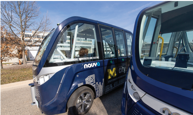
Above: The Mcity Driverless Shuttle project uses two NAVYA Autonom driverless electric shuttles to transport students, faculty, and staff on a non-stop one-mile route on U-M’s North Campus.
