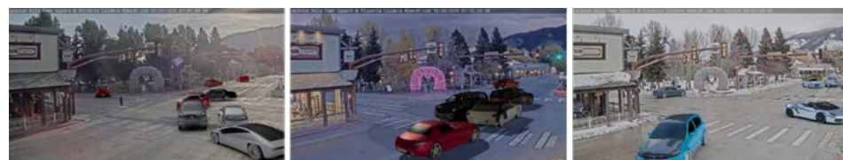
Figure 4: Simulated vehicles with known locations and orientations under diverse weather conditions inserted to help to train our ANN to achieve high perception accuracy.
