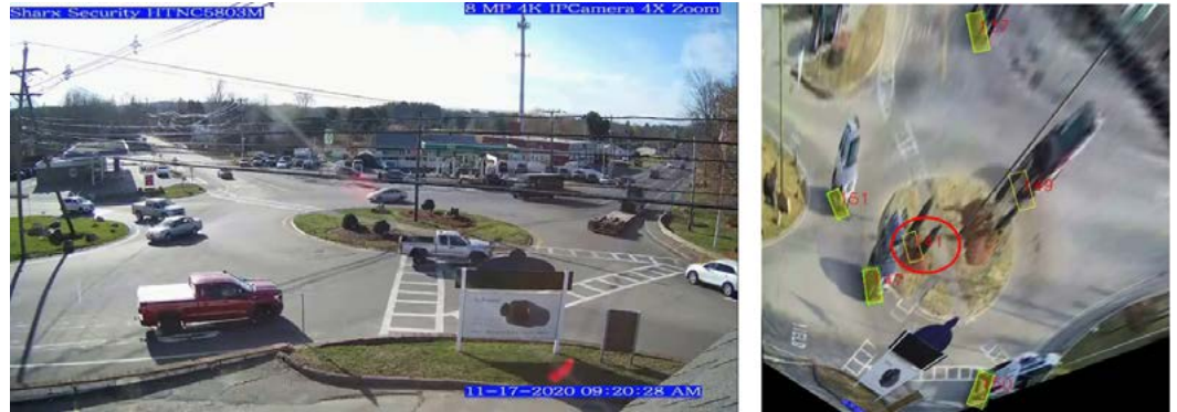
Figure 6: Original image (left) and extracted vehicles shown in 2D bounding boxes (the vehicle footprints on the ground) which indicate position and orientation for the roundabout data collection. Sometimes false positive vehicles, such as the image circled in red with ID 141 in the right photo, need to be filtered out by pixel locations.
